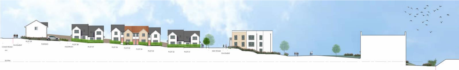
4-4 FACING NORTH – SHOWS GROUND LEVEL FALL TO EAST AND BUILDING HEIGHTS INCREASING
